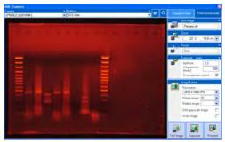
Control of the ImageSystems Felix 1000/2000 With the biostep software argusX1®, all essential functions of the system cameras Felix 1000/2000 can be directly controlled via PC: live-image, zoom, focus, exposure time (integration time), aperture, exposure automatic, white adjustment, ISO value, image resolution.
