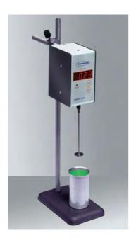
The gelation timers of the GT series are used for the analysis of changeable viscosities of samples. Therefore, these measuring units are often used for quality tests of polymeres, laquers, adhesions and many other liquid multi-component systems.
