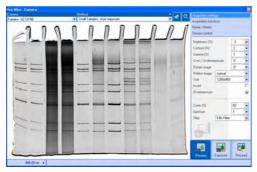
Control of the ImageSysteme Felix 5000/6000/7000 With the biostep software argusX1\*, the following functions of the system cameras Felix 5000/6000/7000 can be directly controlled via PC: live-image, exposure time (integration time), brightness, contrast, gamma, amplification, exposure automatic, image resolution.
