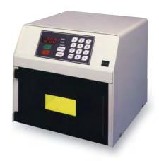
Safety is a major consideration and therefore, the door of the crosslinker is safety interlocked against opening during operation and the observation window in the door is UV-blocking.
