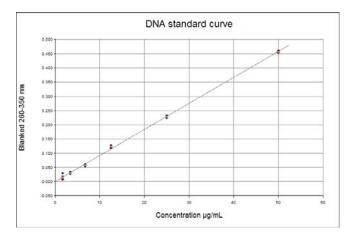
5  $\mu$ L of herring sperm DNA in concentrations ranging from 1.7 ug/mL to 50 ug/mL in replicates of 8 was pipetted into a NCL 96-well IMAPlate and read at 260 nm and 350 nm in a Synergy 4 Hybrid Microplate Reader and (Abs260 – Abs350) is used for this plotting. All data was blanked against an average of 8 wells of deionized water.
