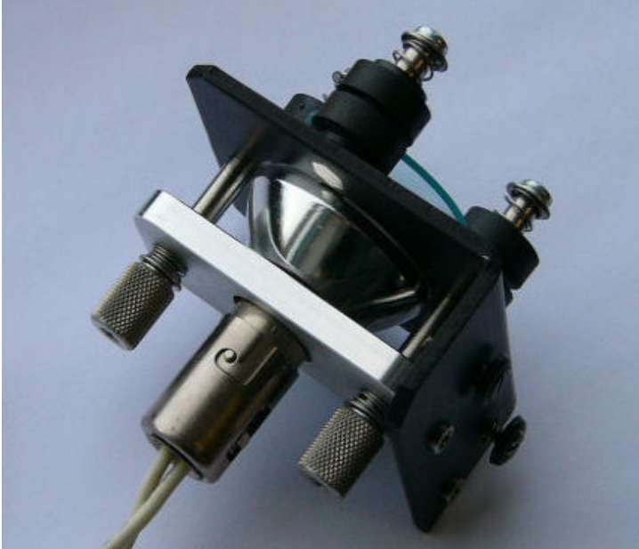
Figure 10: New lamp hardware for the ELx808, assembled (Lamp Assembly 1)
