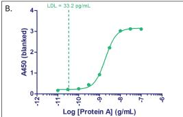
Figure 3. Protein A Standard Curve. A) AlphaLISA Protein A Assay. A12-point dilution series of the positive control was prepared ranging from 100,000 - 0.3 pg/mL was prepared. Twelve background points were used to calculate LDL. B) Protein A ELISA Assay. A 9-point dilution series of the positive control was prepared ranging from 100,000 – 10 pg/mL. Twelve background points were used to calculate LDL.
