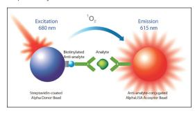
Figure 1. Assay schematic for AlphaLISA homogeneous proximity assay principle for the detection of analyte in biotherapeutic products. Upon excitation, the AlphaLISA donor bead generates singlet oxygen molecules. If the acceptor bead is in close proximity due to the creation of a sandwich immunoassay, the singlet oxygen molecules will trigger a cascade of energy transfer in the acceptor bead, resulting in a sharp peak of light emission at 615 nm.
