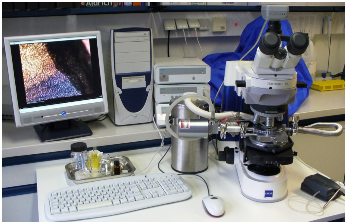
Pic. 2-1: Freeze-dry microscopy equipment (Axiolmager.A1)
