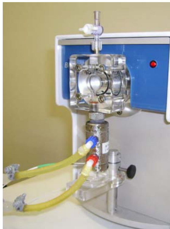
Pic. 2-4: Set-up of the VILASTIC Viscoelasticity Analyzer and of the connected chiller unit
