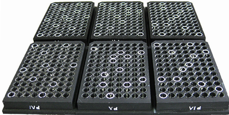
Figure 2.7: Set-up for sublimation tests with the Freeze Drying System. Tubes with white rim are tubes selected for weighing before and after each run. One half of the tubes selected for weighing was placed in edge positions, the other half was placed in centre positions. Positions of selected tubes differed from one block to the next. Vials in block V are not correctly placed in the picture.
