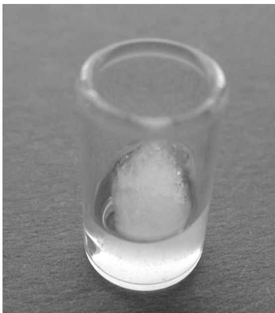
Figure 3.36: Ice core in a single tube of the Freeze Drying System TM photographed after conduction of a sublimation test. The ice has completely lost contact to the tube wall. The temperature of ice and tube at the time the photograph was taken was approximately 0 °C to minimise fogging of the glass. Note that at this temperature, some of the ice has already melted.
