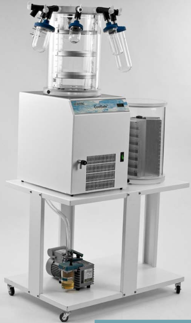
Chamber CC300-8V with shelves and manifold combined.
