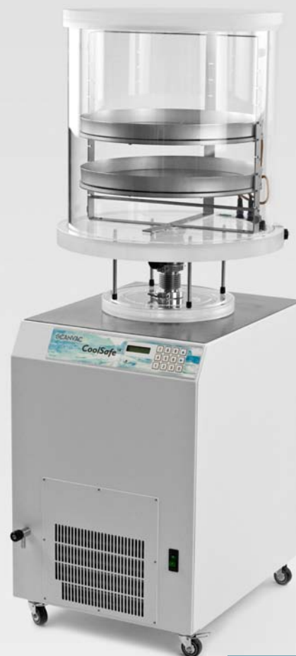
Large condensers can facilitate large chambers.
