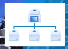
USB networking can be used to connect and drive up to three further satellite thermal cyclers.
